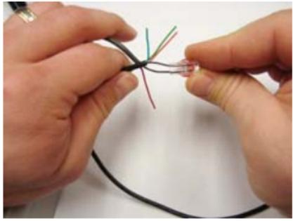
Figure 10 Seating Connector Wires
