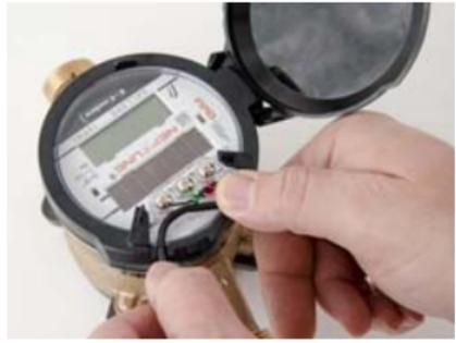
Figure 4 Routing the Wire
