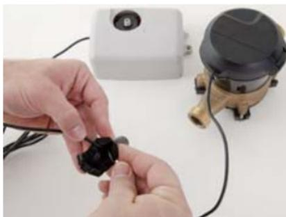
Figure 15 Gray Wires in Slot
