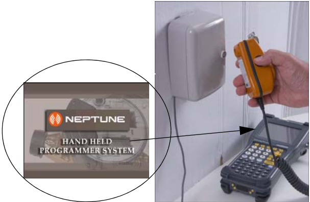
Figure 6 Neptune CE5320 Handheld with Field Programmer Software
