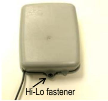
**Figure 2 Wall MIU Main Housing**
