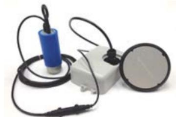
Figure 5 Leak Spy MIU Connected
