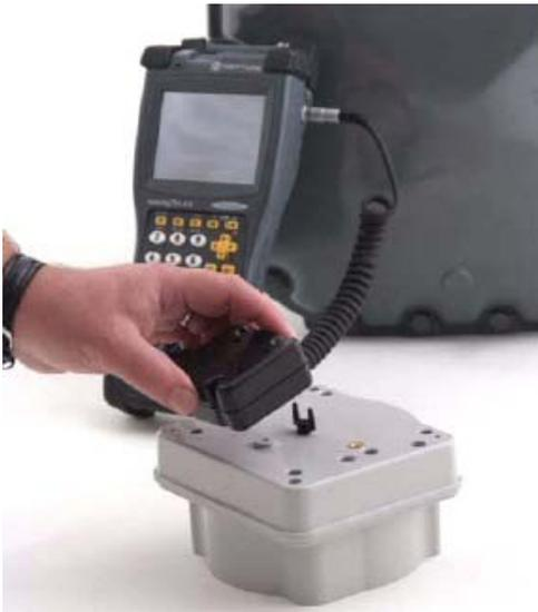
Figure 49 CE5320 Handheld with Programming Mouse
