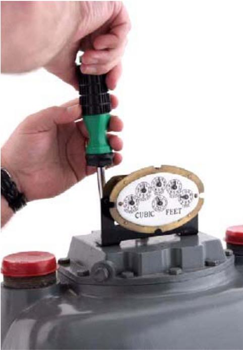
Figure 48 Removing Index Mounting Screws
