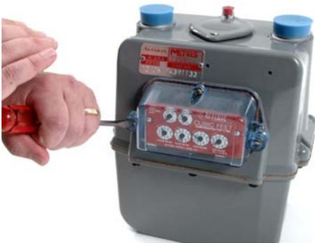
Figure 27 Puncturing and Removing Tamper Plugs
