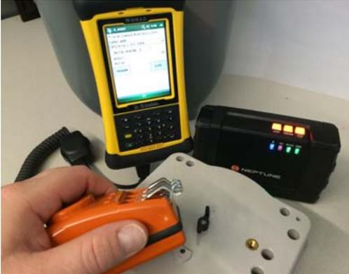
Figure 50 Trimble Nomad, R900 BCT, and USB Programming Mouse
