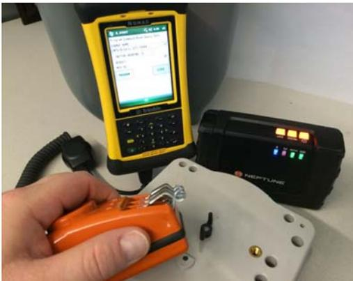
Figure 38 Trimble Nomad, R900 BCT, and USB Programming Mouse
