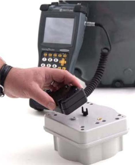
Figure 37 CE5320 Handheld with Programming Mouse
