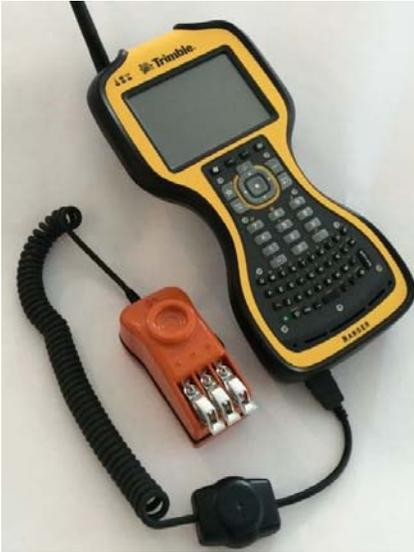
Figure 39 Trimble Ranger with USB Programming Mouse
