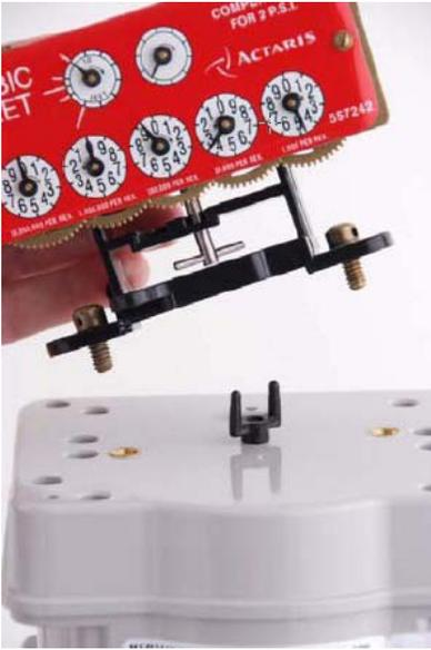
Figure 67 Placing the Gas Meter Index on the R900G
