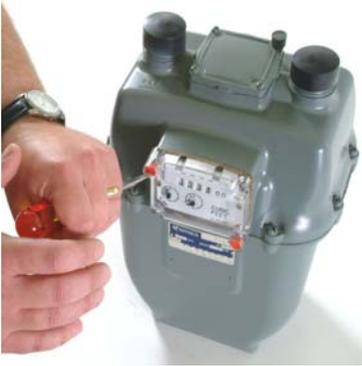
Figure 13 Puncturing and Removing Tamper Plugs
