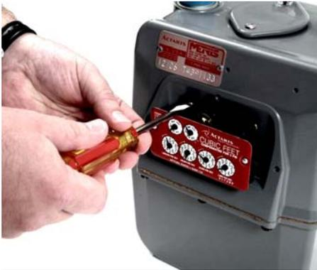
Figure 29 Removing Index Mounting Screws
