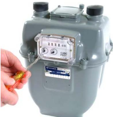
Figure 14 Removing Lens Mounting Screws
