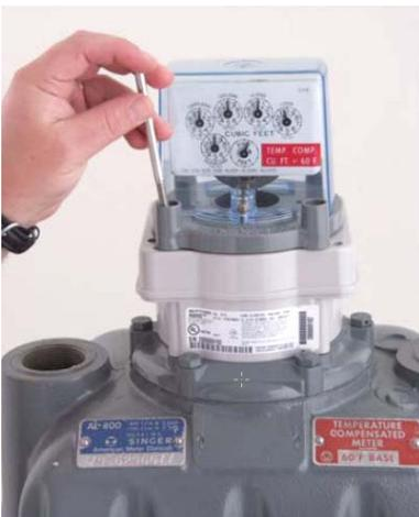
Figure 43 Placing Screws Used to Secure the R900G to the Meter Casing
