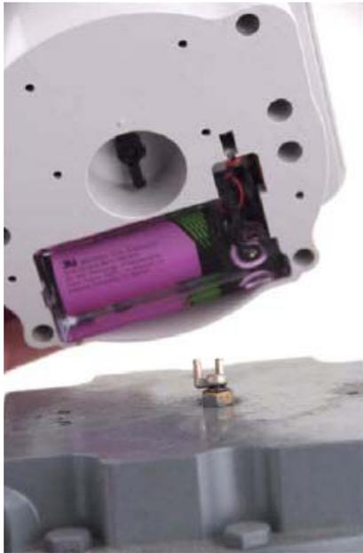
Figure 52 Placing the R900G on the Gas Meter Casing
