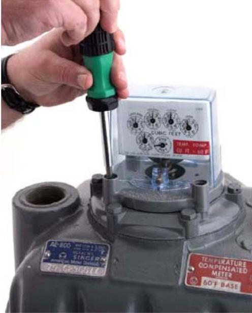
Figure 35 Removing Index Mounting Plate Screws
