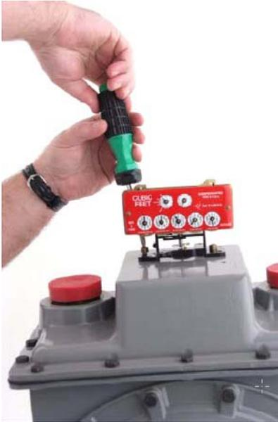
Figure 61 Removing Index Mounting Screws
