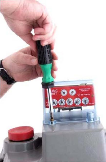
Figure 59 Removing the Index Cover Screws
