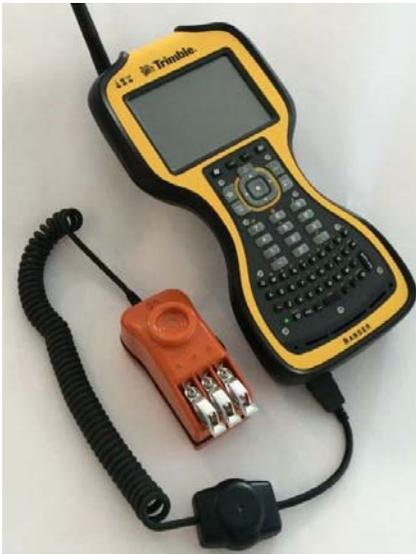
Figure 51 Trimble Ranger with USB Programming Mouse
