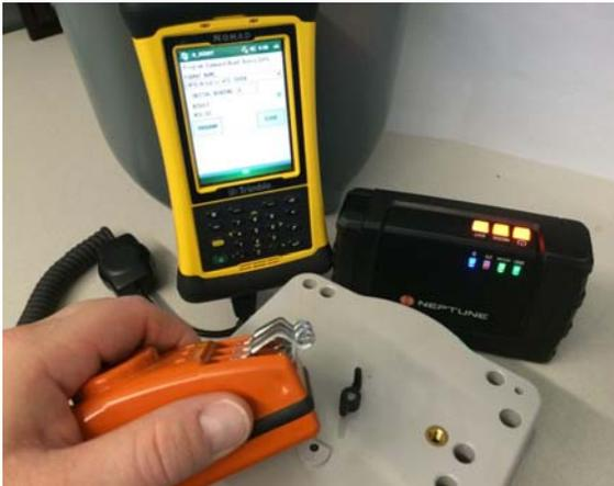
Figure 64 Trimble Nomad, R900 BCT, and USB Programming Mouse
