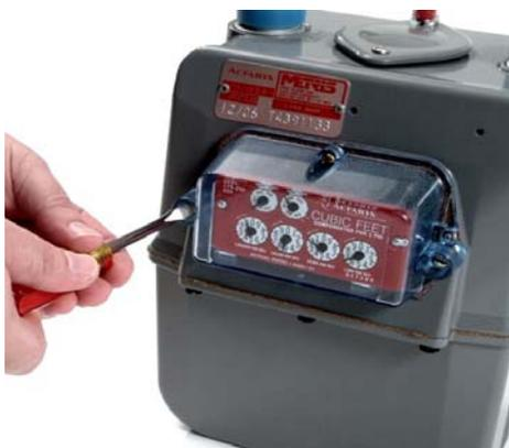
Figure 28 Removing Lens Mounting Screws
