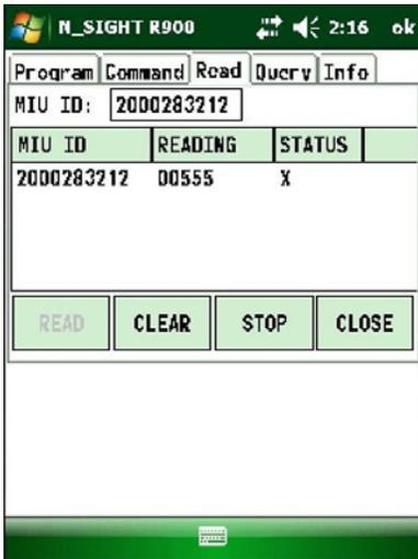
Figure 83 Gas Reading Result Screen
