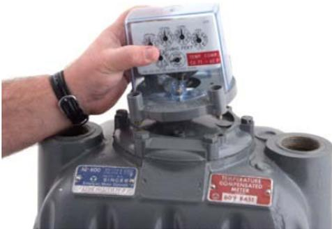
Figure 36 Removing the Index and Mounting Plate
