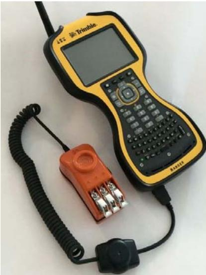
Figure 65 Trimble Ranger with USB Programming Mouse
