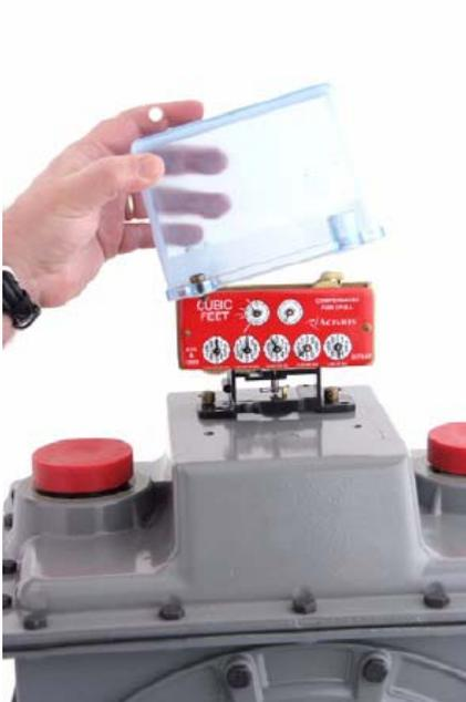
Figure 60 Removing the Index Cover
