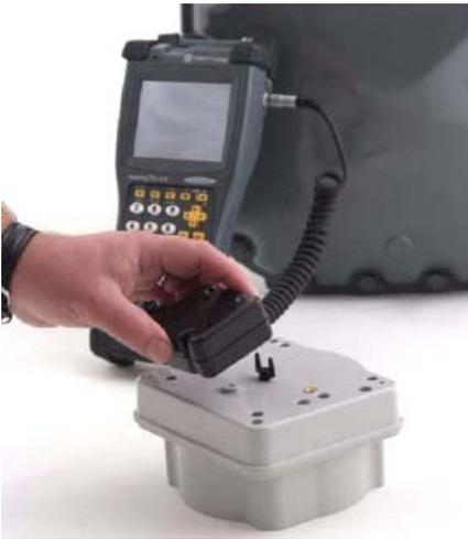
Figure 63 CE5320 Handheld with Programming Mouse
