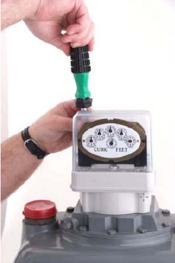
Figure 57 Securing the Index Cover to the R900G and the Meter Casing
