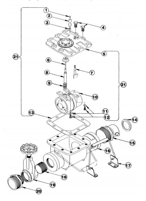
Figure 22 – Representative Breakdown of the Fire Hydrant
