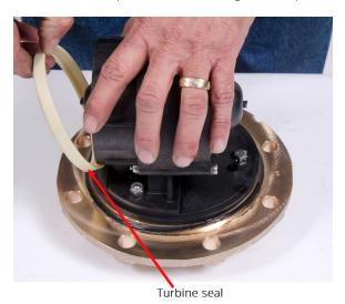
Figure 13 – Turbine Seal
