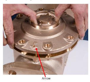
Figure 15 – Top Plate Arrow Aligned with Guide Pin
