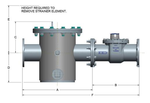
Figure 27 – HP Fire Service Turbine S Dimensions
