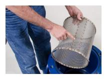
Figure 30 - Checking for Defects
