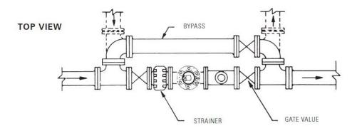
Figure 3 - Recommended Installation - Top View
