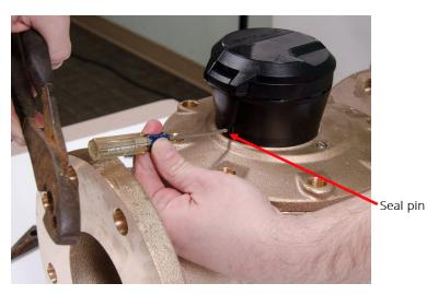
Figure 7 - Tapping the Seal Pin
