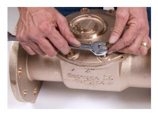
Figure 9 - Removing the Bolts
