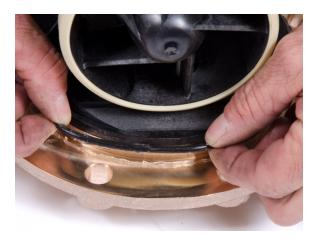
Figure 12 – Inspecting the O-Ring
