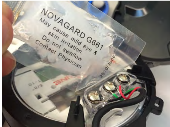
Figure 8 – Application of the Sealant
