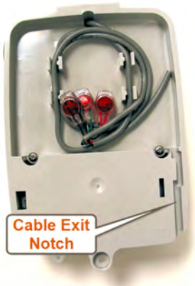
Figure 16 – Cable Exit Notch
