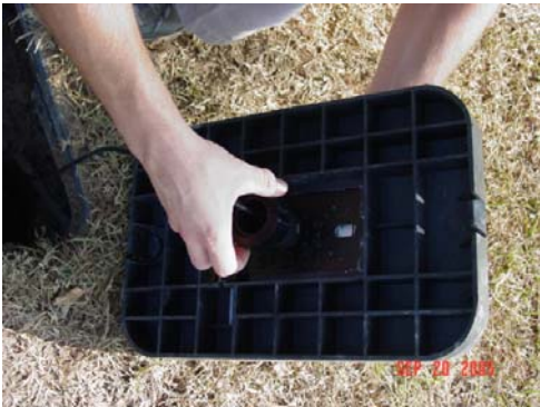
Figure 8 Feeding Antenna Cable
