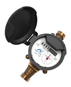
The Neptune® ProCoder™ solid state absolute encoder register features a high-resolution, mechanical sweep hand to detect ultra-low flows as well as monitor direction of flow. The ProCoder's non-contact LED absolute encoding technology ensures the odometer read exactly matches the remote read. It provides a high-resolution, 8-digit remote meter reading along with leak, tamper, and reverse flow flags when connected to a Neptune R900® System endpoint.
