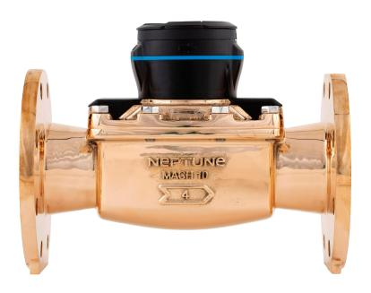
The MACH 10® ultrasonic water meter features solid state ultrasonic technology including a factory-calibrated, replaceable unitized measuring element (UME) with no degradation of accuracy over time. Combined with a corrosion-resistant, lead free, high-copper alloy maincase, the MACH 10 is built to withstand demanding service conditions and deliver sustained accuracy over the life of the meter.
