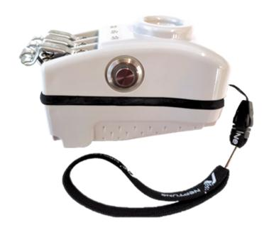
The Neptune Bluetooth Field Programming Mouse provides the capability to program, query, and read Neptune registers with a utility-owned device. The Mouse, used in conjunction with the Neptune® 360™ Field Manager programming application, seamlessly pairs with a smartphone or tablet via Bluetooth to simplify field programming without the need for a third-party tool. Reprogram ID numbers and dial codes, or change the format of a Neptune register with ease.
