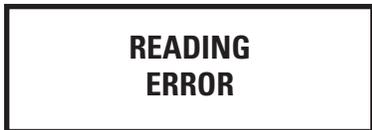
To correct either error condition, position the probe such that proper contact is achieved with the remote. For ProRead and Sensus meters, the trigger must be pulled after making proper contact.
