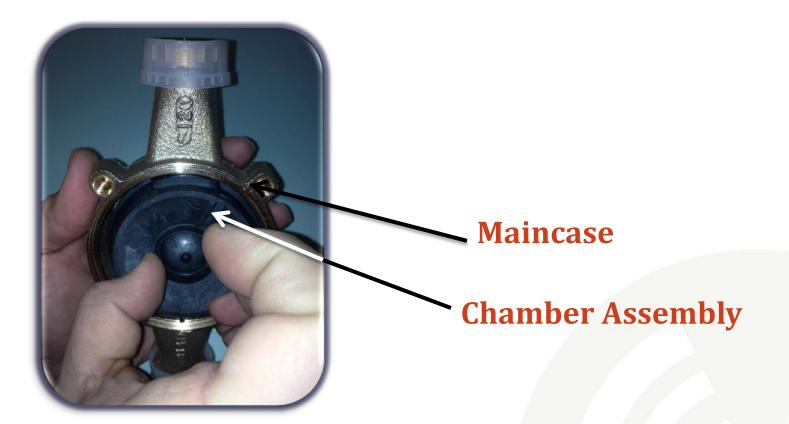
Place chamber assembly into meter maincase. Ensure outlet gasket is facing the outlet of the meter.
