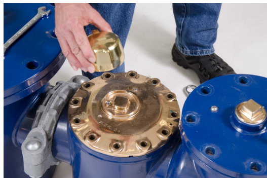
Figure 25 – Removing the Register from the HP Turbine
