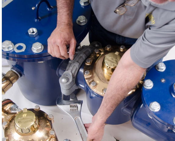
Figure 55 – Removing the Bolts
