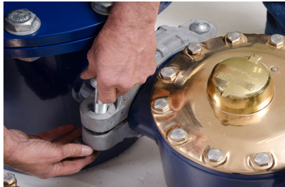
Figure 61 – Tightening the Bolts
