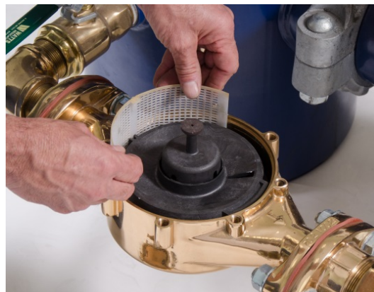
Figure 20 – Inserting the Strainer
