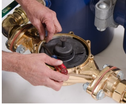
Figure 13 – Removing the T-10® Strainer
