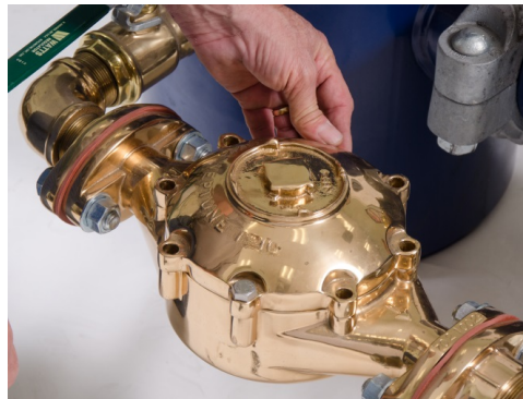
Figure 23 – Reinstalling the Top Plate
