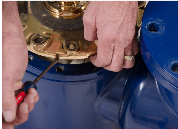
Figure 26 – Removing the HP Turbine Top Plate
