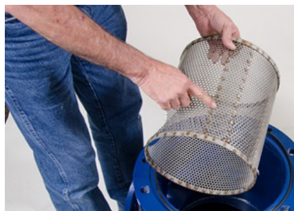
Figure 22 Inspect Strainer Basket
