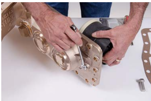
Figure 29 Removing the Lock Nuts
