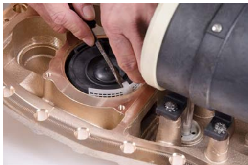
Figure 18 Removing the T-10 Strainer
