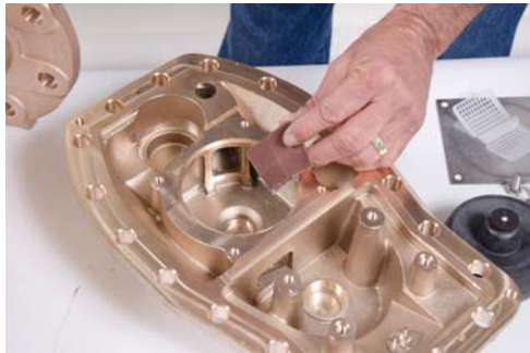
Figure 21 Cleaning Around the Chamber
