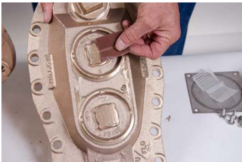
Figure 22 Cleaning Under the Registers
