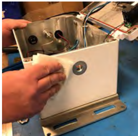
Figure 108 – Clean Antenna Mounting Area
