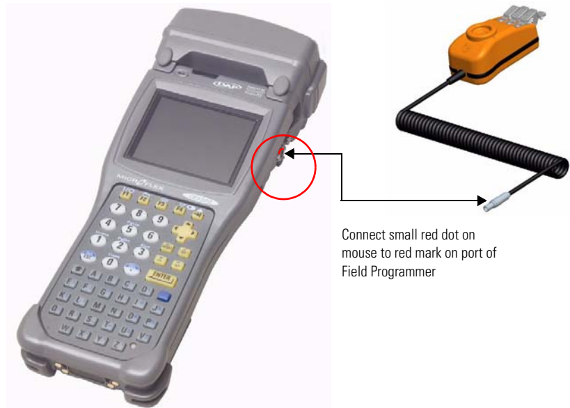
Figure 2.2 Connecting Mouse to Field Programmer
