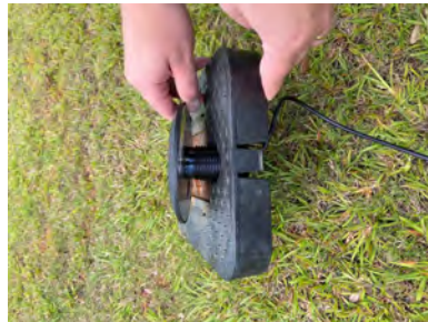
Figure 52 – Inserting the Antenna into the Pit Lid
