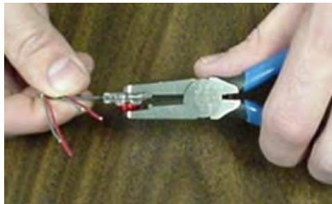
Figure 15 – Crimping the Connector
