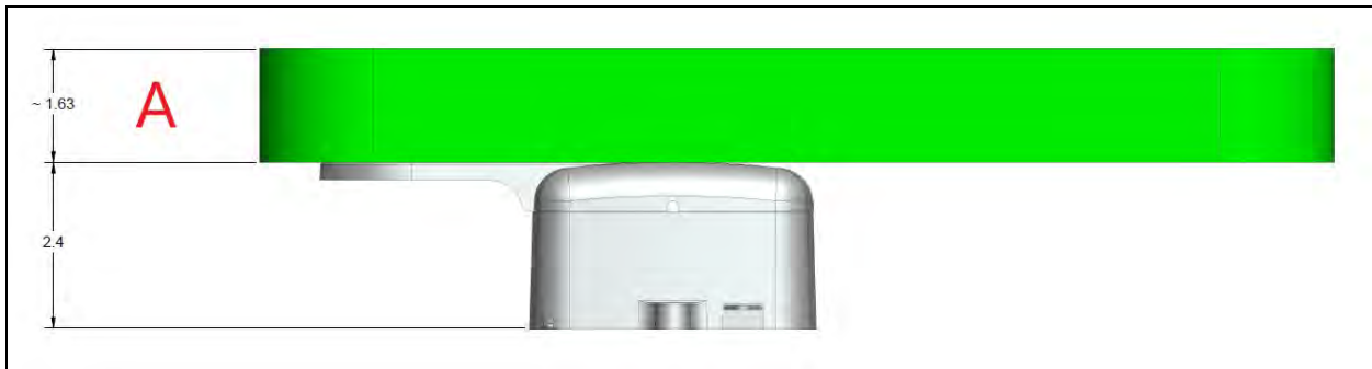
Figure 37 – Pit Cellular Endpoint with Vertical Antenna Clearance
