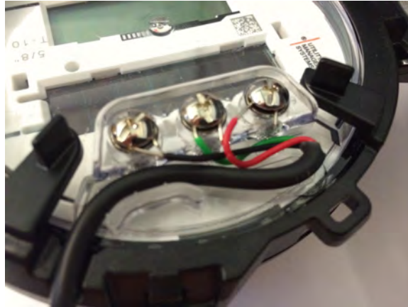
Figure 9 – Cable Threaded Around Strain Relief Posts
