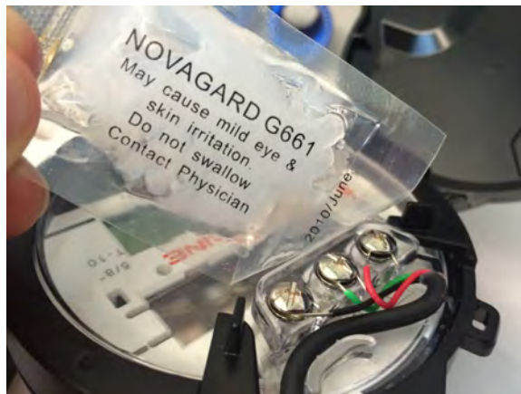
Figure 10 – Application of the Sealant
