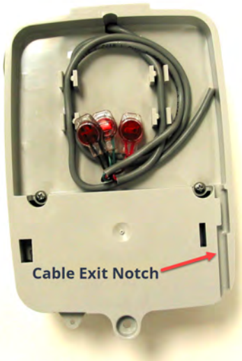
Figure 26 – Cable Exit Notch
