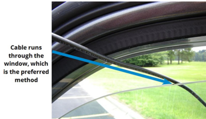
Figure 15 – Antenna Cable Through Window
