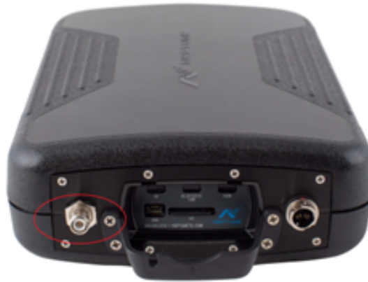
Figure 13 – Mobile Data Collector RF Antenna Connector
