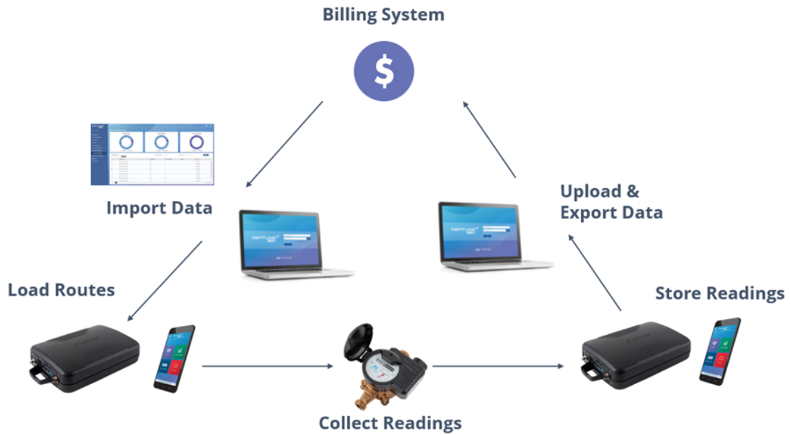
Figure 2 – Mobile Data Collector Meter Reading Operations
