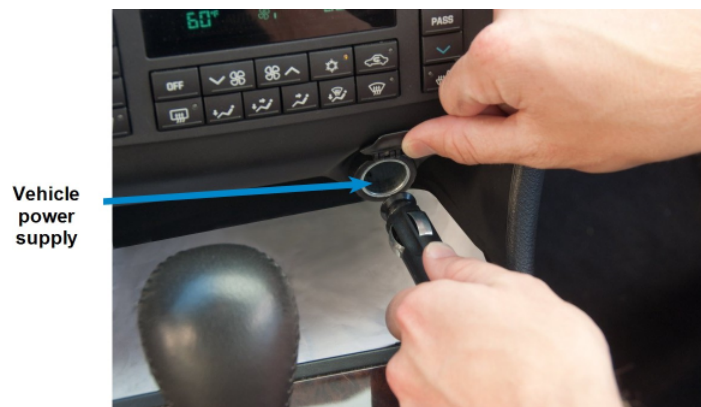
Figure 11 – Power Supply Cable Inserted into Vehicle
